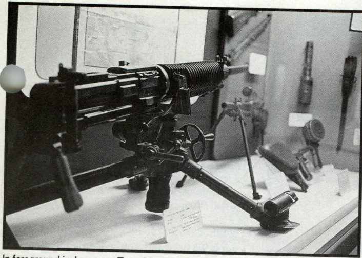
In foreground is Japanese Type 92 Heavy Machine Gun cal. 7.7mm, weight 61 pounds, weight w/tripod 122 pounds, cyclic rate of fire 450-500 rpm. Made by Nambu Armament Manufacturing Co., Tokyo.
