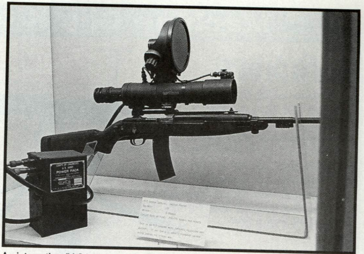
An interesting (U.S.) M-3 Sniper Carbine, cal. .30, weight 5 pounds, cyclic rate 750-775 rpm. This is an M-2 Carbine with infrared telescope and battery. It was the Army's standard sniper rifle during the Korean War.
